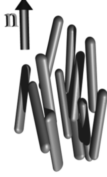
Figure 2.1: Nematic liquid crystals with director orientation \mathbf{n} [74].
